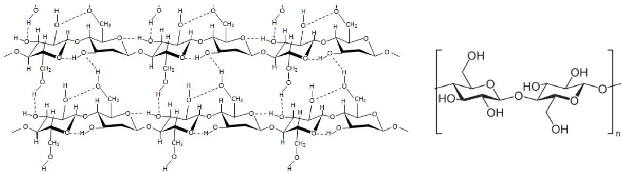
Figure 3: BC network (left) with a close-up of the BC molecular structure [11]
