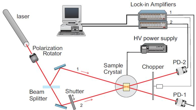
Figure 4: Two-beam coupling experimental setup [4]
