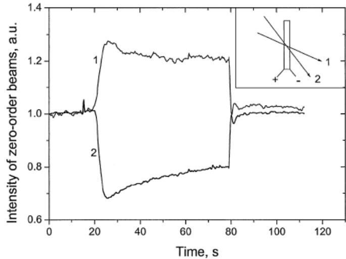
**Figure 6:** Sample data showing the beam coupling within a sample of homeotropically aligned 5CB. A DC electric field is applied at approximately 20 s and turned off at 80 s [1]
