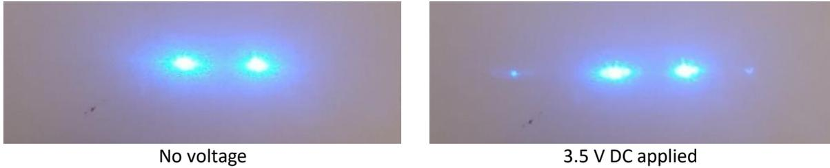
**Figure 10:**  $\pm 1$ st order diffracted beams are observed on the right when a DC voltage of 3.5 V is applied across the 5CB cell.
