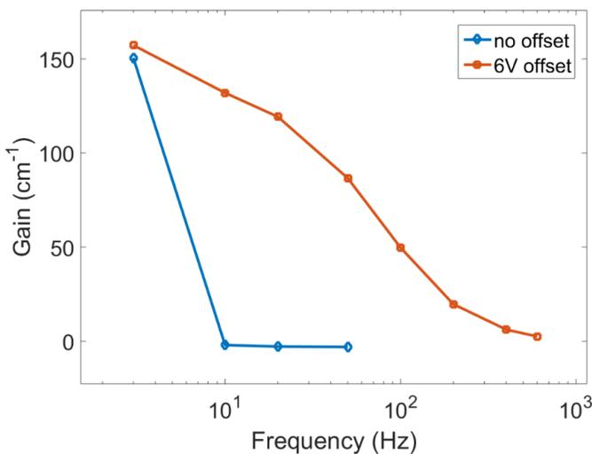
**Figure 12:** Frequency dependence of gain with the application of 40 V<sub>pp</sub> across  $C_{60}$ -doped 5CB cells.
