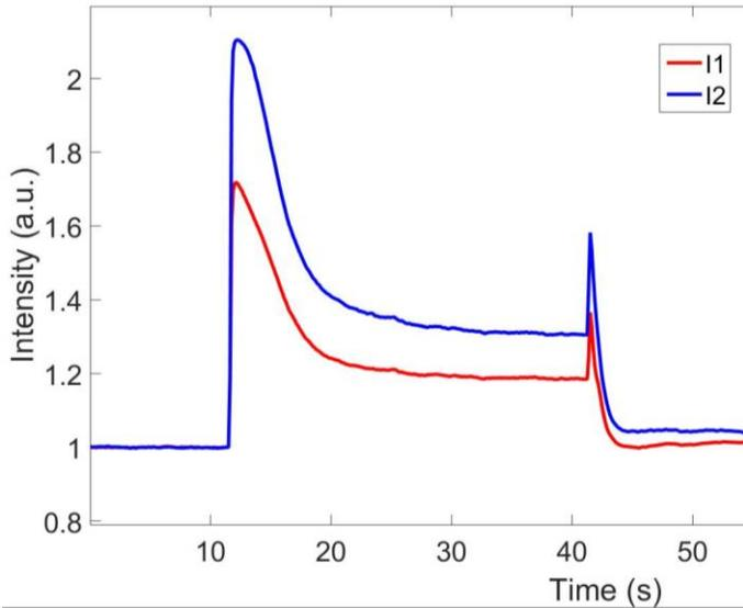
**Figure 11:** Sample beam coupling data. 3.5 V were applied across a  $C_{60}$ -doped 5CB cell sample at 12 s and removed at 41 s. The transients at the beginning and end of the electric field are due to charging and screening [16]
