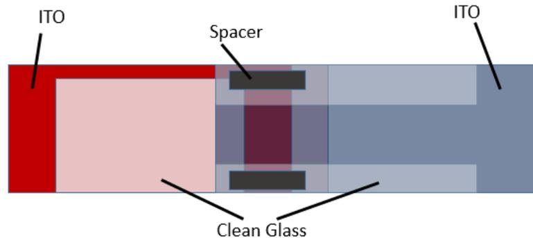
**Figure 8:** C- and T-shape of the ITO for the BC mat samples with one substrate in red and the other in blue.
