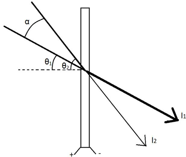
Figure 5: Schematic of beam coupling in the material.  $I_1$  and  $I_2$  are the measured beam intensities,  $\theta_1$  and  $\theta_2$  are the respective incident angles with respect to normal, and  $\alpha$  is the mixing angle. In this case,  $I_1$  is intensified and  $I_2$  is diminished.
