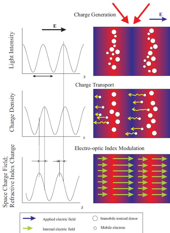
**Figure 1:** Photorefractive grating formation. From top to bottom: charge photogeneration, charge transport, and refractive index modulation [4]
