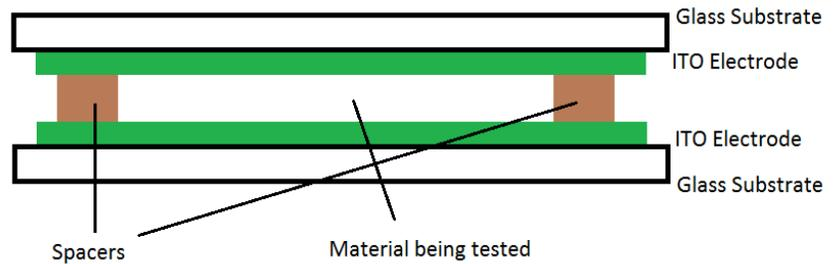
**Figure 7:** Side-view of a basic test sample
