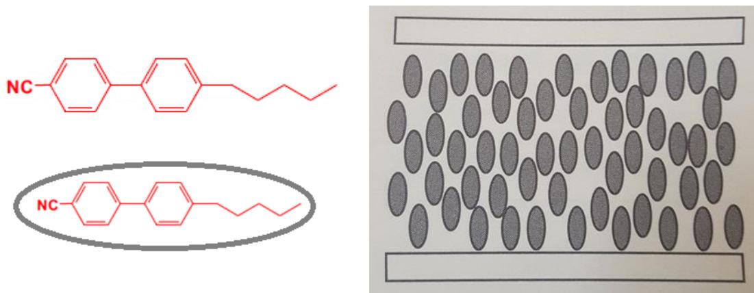
**Figure 2:** Molecular structure of 5CB (top left) [4], 5CB approximated by elongated ovals (bottom left), and the 5CB homeotropically aligned nematic phase structure (right) [7].
