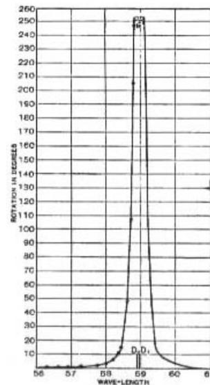
**Fig. 5-7.** Rotation (in degrees) of plane of polarization vs. wavelength in sodium vapor.
